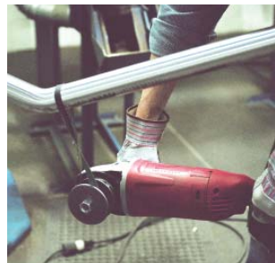
Finishing Pulley in use with 6000 RPM, 9" Grinder, 15 amp.
