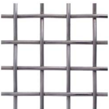
Stainless BWP-278 Open Area: 70.1% Weight: 1.70 lbs/sqft Opening Limitation: .838" Overall Thickness: .320" Aspect Ratio: 1.00:1
