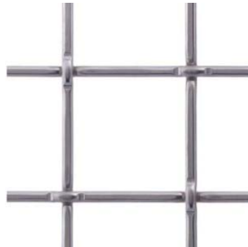
Stainless BWL-62 Open Area: 81.7% Weight: 1.20 lbs/sqft Opening Limitation: 1.810" Overall Thickness: .380" Aspect Ratio: 1.00:1
