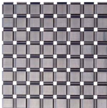
Stainless BWS-13 Open Area: 6.6% Weight: 3.67 lbs/sqft Opening Limitation: .125" Overall Thickness: .125" Aspect Ratio: 1.00:1
