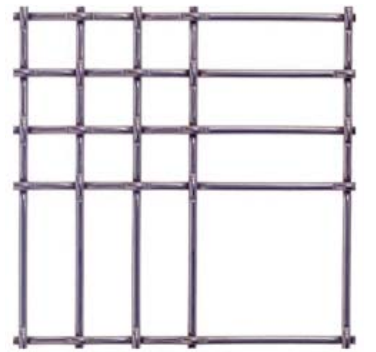
Stainless BWM44-2 Open Area: 77.4% Weight: 1.04 lbs/sqft Opening Limitation: 2.100" Overall Thickness: .255" Aspect Ratio: 1.00:1
