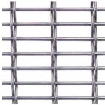
Stainless BWM12Z-17 Open Area: 61.7% Weight: 2.12 lbs/sqft Opening Limitation: .471" Overall Thickness: .390" Aspect Ratio: 2.67:1
