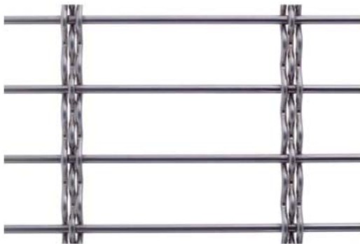
Stainless BWM13Z-7 Open Area: 76.9% Weight: 1.30 lbs/sqft Opening Limitation: 1.042" Overall Thickness: .375" Aspect Ratio: 3.25:1
