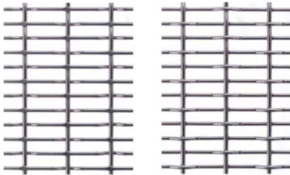
Stainless BWFpz-46 Open Area: 64.0% Weight: 1.36 lbs/sqft Opening Limitation: .213" Overall Thickness: .215" Aspect Ratio: 3.00:1
